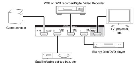
Connect your components to the appropriate jacks. The default input assignments are shown below.
